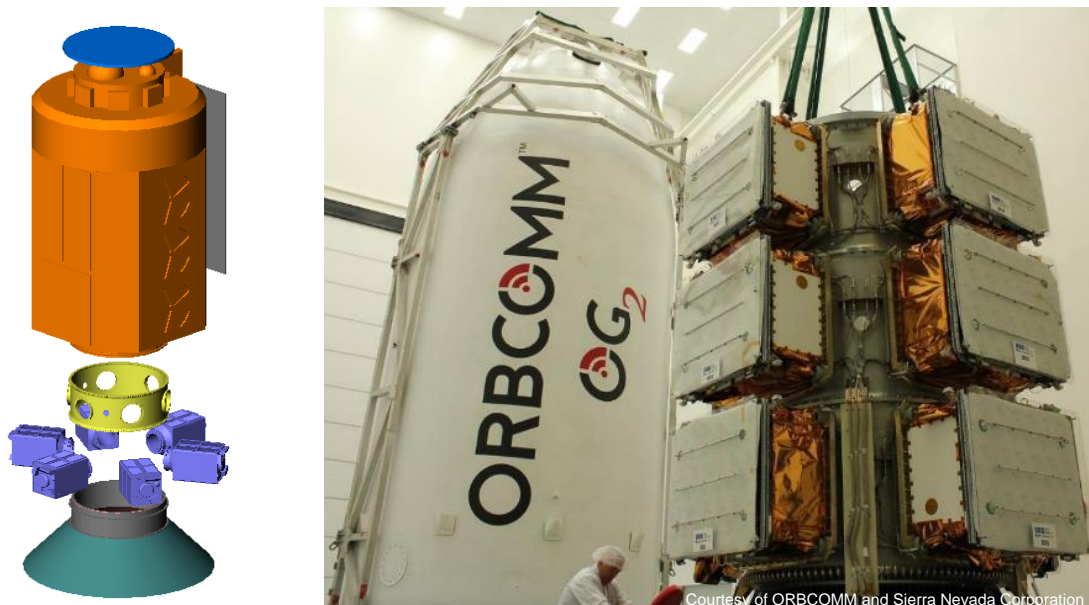
Figure 2. Left, ESPA and auxiliary payloads launching with primary spacecraft Right, ESPA stack for ORBCOMM OG2 spacecraft
